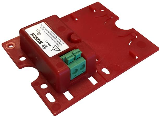
This end-of-line device is a reliable solution for loudspeaker line integrity supervision, which is a requirement for emergency sound systems. It is connected at the end of a loudspeaker line, after the last loudspeaker of a series of looped-through loudspeakers.
