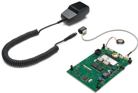
The basic call station kit is an open frame call station to create dedicated full custom operator panels for PRAESENSA Public Address and Voice Alarm systems. It has the same functionality as the PRA-CSLW, but without LCD user interface to facilitate easier mounting in operator desks or in wall-mounted fireman's panel enclosures.
