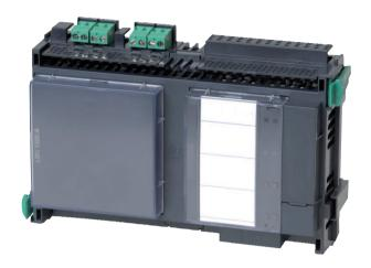
This module allows the connection of an LSN loop with up to 254 LSN improved elements with a maximum line current of 1500 mA or with up to 127 classic LSN elements, with a maximum line current of 300 mA.
