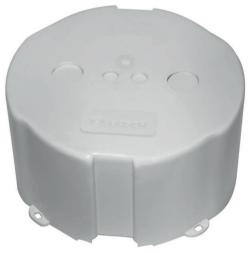
The back box is made from ABS material and is color matched with the ceiling loudspeakers. The unit has knockout holes and is supplied with cable glands. The unit can only be used as a back cover for LBD0606/10 and LCZ-UM12-IN ceiling loudspeakers. The back cover can be fitted to the ceiling loudspeaker frame by using the supplied self tapping
