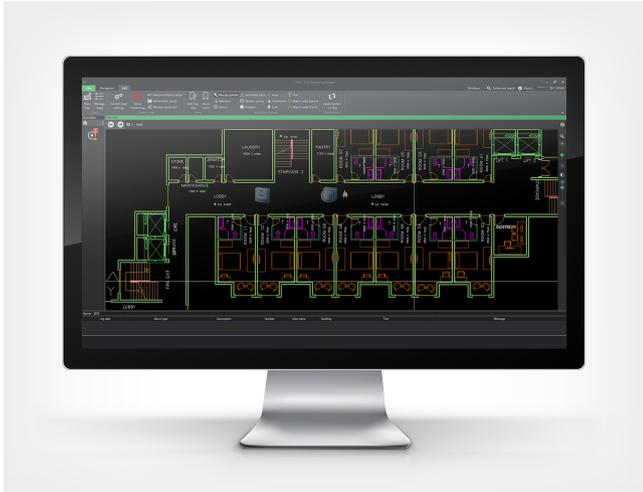
The Fire Monitoring System is a graphical user interface for displaying and monitoring small to medium fire alarm systems with up to 10000 detection points. It is compatible with AVENAR panel 8000, AVENAR panel 2000, FPA-5000 and FPA-1200.
