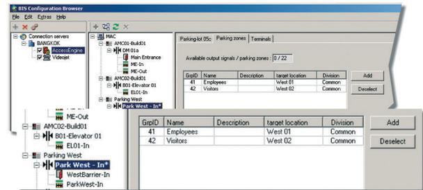
This feature allows the definition and use of the door model "parking lot" which contains the control of two barriers for entrance and exit and their traffic lights, which prevent access when the lot has reached maximum capacity.
